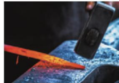
Figure 25.13 The hotter part of the metal is radiating strongly across the visible part of the spectrum, and appears yellow. Cooler parts emit most of their light in the red part of the spectrum.
